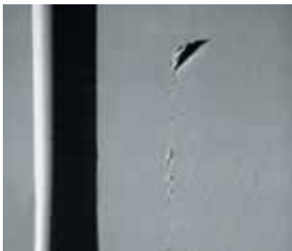
Figure 2 - SEM at 50X magnification shows intimate contact of the internal hex implant at both the beveled implant/abutment interface and the hexagonal engagement area.
